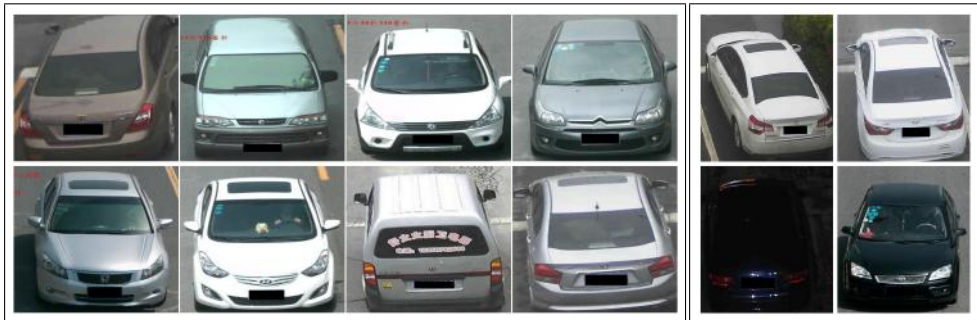
Figure 5: Qualitative evaluations of vehicle model classification. (Left) : Correctly classified vehicle images with large visual appearance similarity between different model classes. (Right) : Misclassified vehicle images due to extreme illumination conditions.
